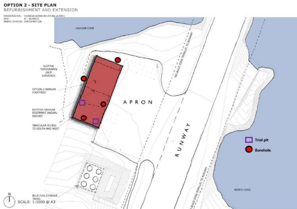
Figure 4-13: Option B (Formerly Known as Option 2) Borehole and Trial Pit Locations
