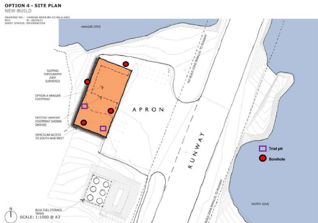
Figure 4-14: Option C (Formerly Known as Option 4) Trial Pit and Borehole Locations
