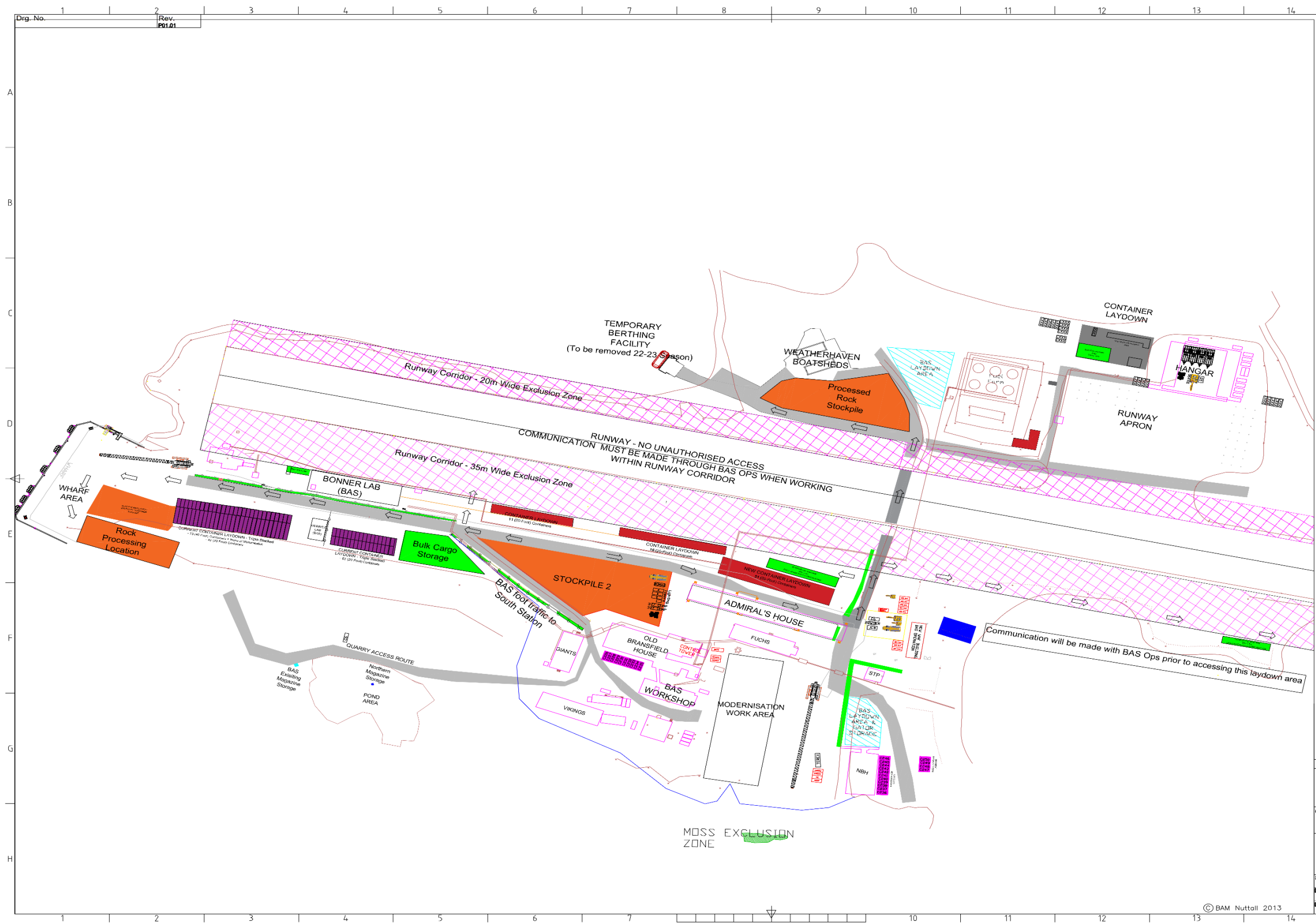
Figure 4-19: Site Layout Plan Including Main Laydown and Storage Areas, BAM 2022
