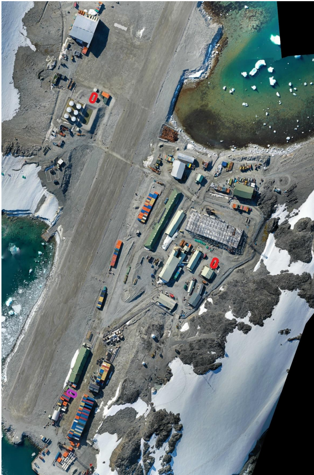
Figure 4-2: Proposed areas for the two 2,000-litre storage tanks (red) and the proposed position for the 950-litre tank (purple), BAM 2022
