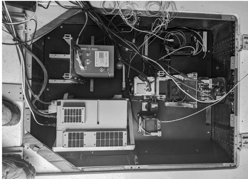
**Figure 4.1:** A series of broadband and hyperspectral imagers installed in the viewing hatch of the BAS Twin Otter aircraft by the NAEO. Each sensor is generally operated by an independent computer that has its own control and data storage requirements. Note boots at far left for scale. See Figure 2.1 for the actual aircraft this installation is hosted within.
