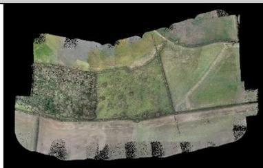
Photogrammetric orthomosaic generated from Matrice 300RTK
