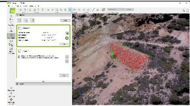
Estimating volume of mine waste from the 3D model
