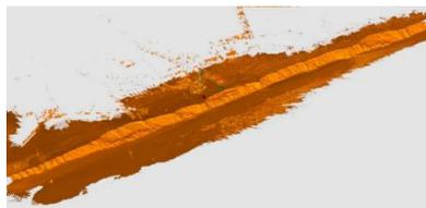
DEM created from combined TLS and UAS LiDAR
