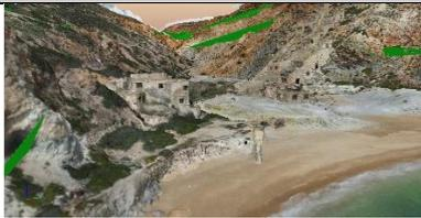
3D model for the Sulphur deposit generated from the RGB imagery. Green surfaces are interpreted paleo water table.
