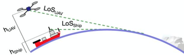
Fig 5: Line of Sight from ship vs. UAV
