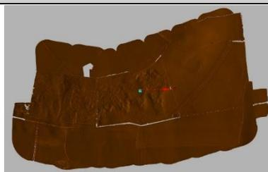
DTM generated from Matrice 300RTK showing landslide area beneath trees
